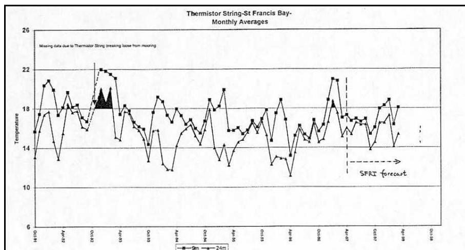
**Fig 5:** SST and bottom temperature measurements collected at the Kromme Bay offshore mooring (stn 9). Under normal easterly wind patterns, a strong, semi-permanent thermocline is set up in coastal waters. During summers of low easterly intensity (ie El Niño), the thermocline becomes weak, resulting in higher bottom temperatures.
