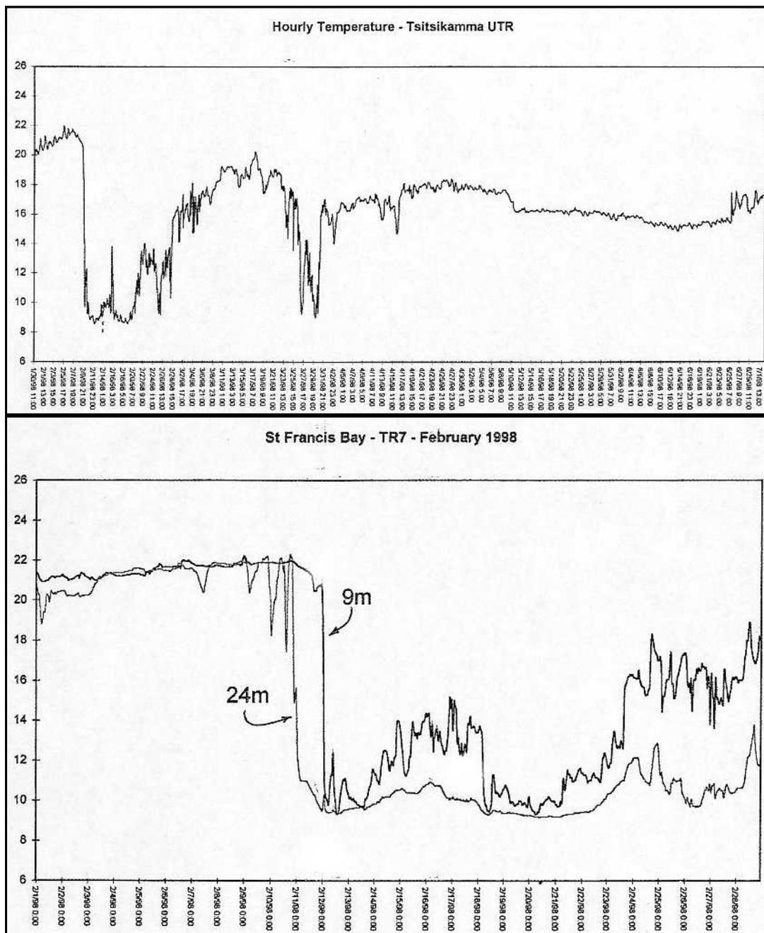
Fig 6: The significant second BMP in February and March abruptly “switched on” the easterly wind-upwelling process. This is clearly seen in (upper) the hourly temperature record for the Tsitsikamma underwater temperature recorder (UTR), 10 m depth, and (lower) at the Kromme Bay mooring (stn 9), 24 m depth. Notice the temperatures were restored to typical SST values by end March.
